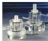
Gas-tight chambers in a Clark electrode
